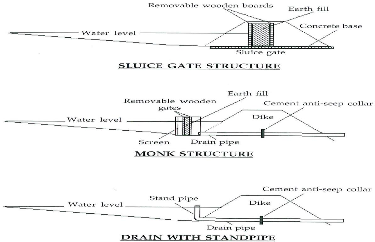
Figure 15: Cross sections of three structures used for draining ponds.
