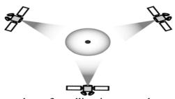
Figure shows 3 satellites in geosynchronous orbit each 120 degree from one another so that whole earth can be covered
