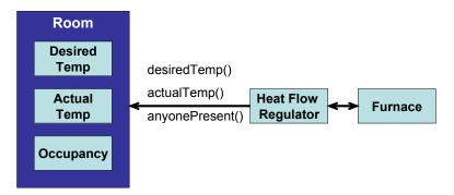
This happened because in the first case intelligence is distributed while in the second case it is encapsulated. However, the control is still centralized as the Heat Flow Regulator has the control logic that first analyses the values from different queries and then makes a decision about turning the furnace on of off. We can improve the situation even further by delegating this responsibility to the Room object as shown below.
