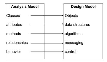
Translating the analysis model into a design model during object design
