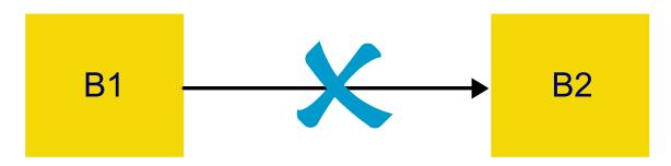
There must be an intermediate process which should transform data received from one external entity and then send the transformed data to the other external entity. As we have already described that data flow diagrams should be used to depict processes that transform or process data. Simple data movement from one entity to another should not be described using data flow diagrams.
