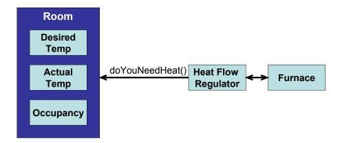
By doing that we reduce coupling even further because now we have made Room more cohesive by putting the function with the related data and have thus reduced the number and types of messages being sent from the regulator to the room.
