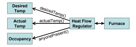
In this case, the room is not encapsulated as one entity and three different objects namely *Desired Temp, Actual Temp,* and *Occupancy* maintain necessary information about a room. In this case the Heat Flow Regulator has to communicate with three different objects.
