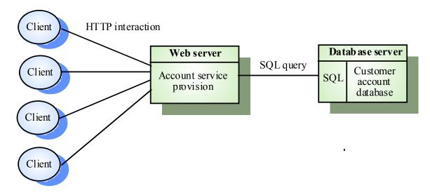
N-tier architecture generalizes the concepts of 3-tier architecture. In this case the system architecture may have more than 3 layers. That is, in n-tier architecture, in order to increase performance, we may distribute the application over different servers by putting different subsystems on different servers.
