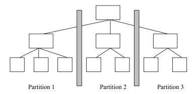
Vertical partitioning divides the application from a decision making perspective. The architecture is partitioned in horizontal layers so that decision making and work are stratified with the decision making modules residing at the top of the hierarchy and worker coming at the bottom. This partitioning is also known as factoring and the general model is depicted in the following diagram.
